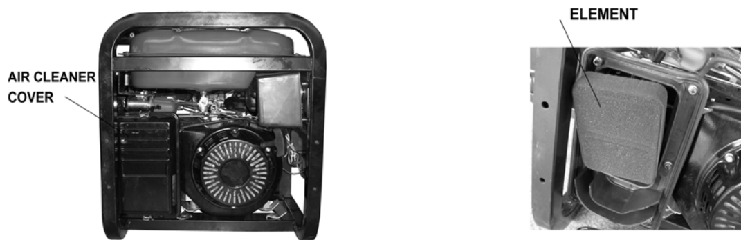
Figure 15- Removing the air cleaner casing.
